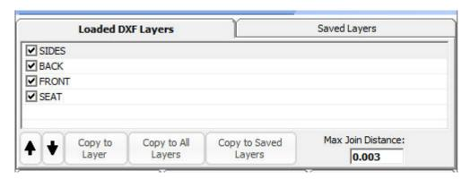
Since a drawing may contain information that you don't necessarily want converted to G-Code such as a title block or dimensions, you can turn these layers off by unchecking the box next the layer name. When layers are turned off or on the viewport will update to display just the layers that are on.
